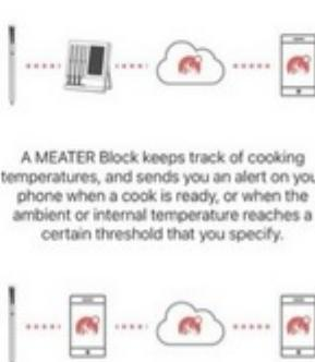
A MEATER Block keeps track of cooking temperatures, and sends you an alert on your phone when a cook is ready, or when the ambient or internal temperature reaches a certain threshold that you specify.
